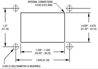
\* The two dimensions marked with an \* specify the minimum recommended panel cutout opening for ACM20 power meters. Space permitting, the larger dimensions noted (0.87in., and 1.426in.) should be used. The panel opening must be centered vertically and horizontally between the four 0.093 (2.362mm) diameter holes.
