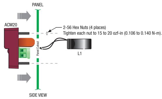
Figure 5. Panel Installation
