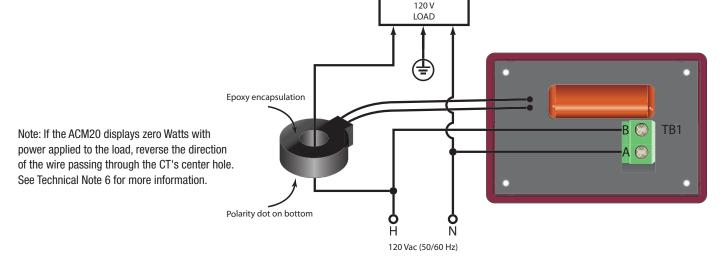
Figure 1. Wiring diagram for 110/120V single phase systems
