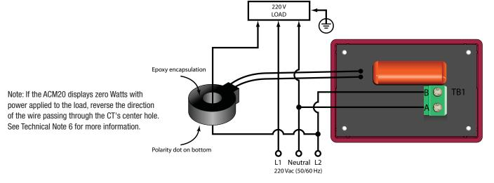
Figure 4. Wiring diagram for 220/240V systems with neutral (monitoring L2)
