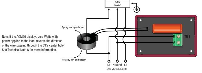
Figure 3. Wiring diagram for 220/240V systems with neutral (monitoring L1)
