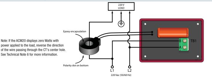
Figure 2. Wiring diagram for 220/240V systems with no neutral
